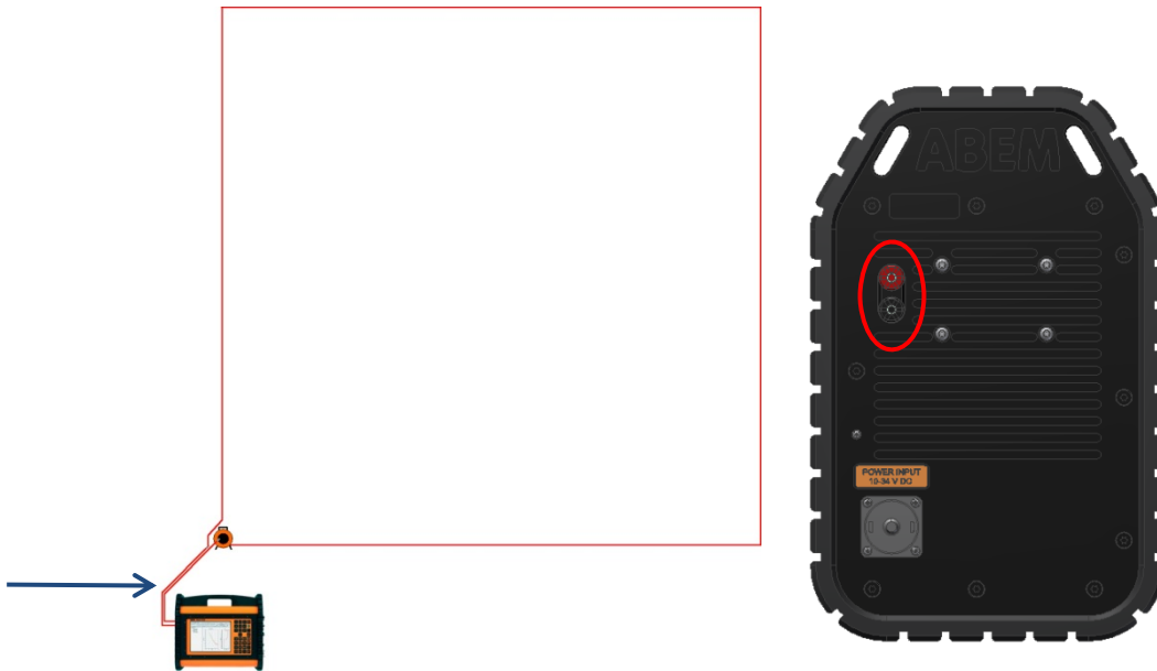
Figure 9. Transmitter loop is connected using the 3 meter lead-in cable. This permits the instrument to be placed 3 meters away from the transmitter loop and the electromagnetic field it generates.
