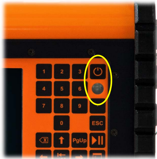
Figure 18. The location of the power on/off button and power indication lights on the WalkTEM
